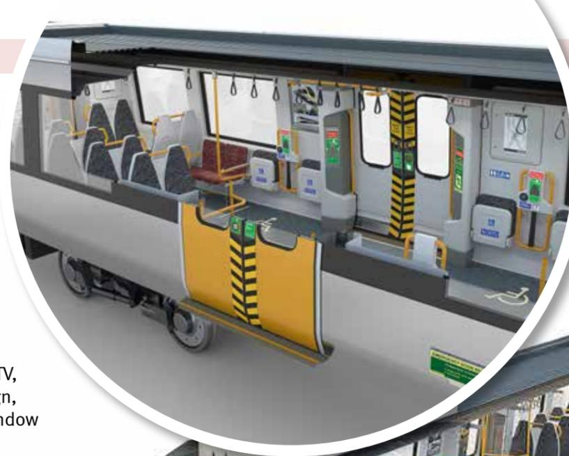
12 accessible areas equipped with velcro restraining straps to secure mobility aids, bicycles or prams
